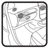
① Filter located behind glove box under dash board.
