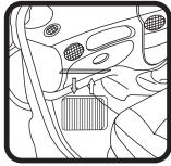
③ Pull dirty filter down to remove, push new Ryco filter up in to housing. Check for correct fitment.
