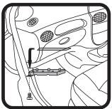
② Undo bolt, slide cover towards front of car and pull down to remove.
